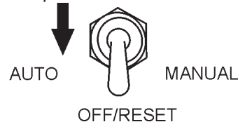
Figure 55. MPEC Control Switch (Off/Reset)
